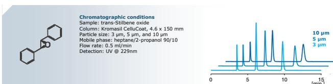
Figure 1. Consistent retention and selectivity independent of particle size
